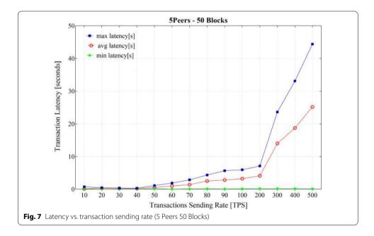
Hence, there was a need to deploy a smaller block size with a low transaction rate for IoT applications to have lower transaction latency. In contrast, higher transaction rates needed larger block sizes to achieve higher throughput and lower transaction latency (the results of latency measurements for various block and batch sizes are presented in Figs. 6 and 7). It happened mainly due to the increasing waiting time for transactions in the ordering services.
