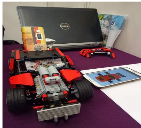
Figure 5. Prototype set-up for the wheel, GUI and mobile applications
