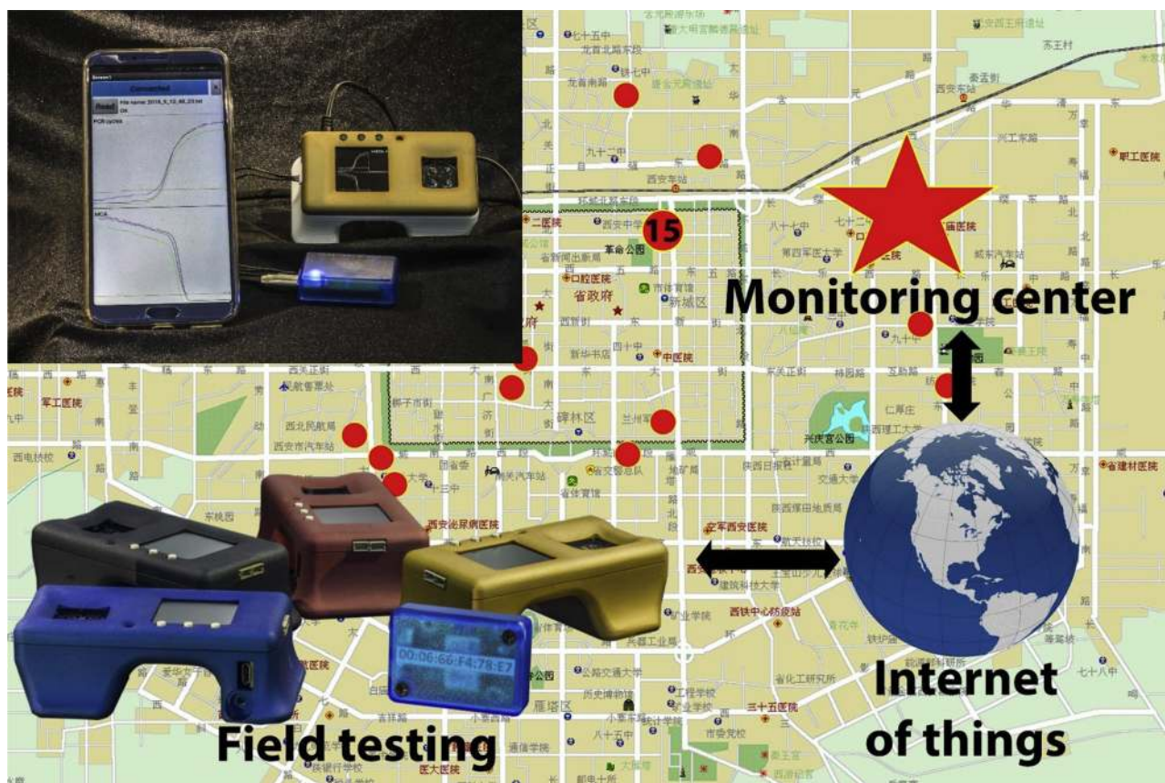
Fig. 4. IoT PCR as a part of IoT. A mock-up test showing the hypothetical spread of DEVN in Xi'an. Red dots represent individual cases; more cases in the vicinity of each other are clustered into a larger dot with the number of cases the dot represents. (top left inset) The results from a single run shown on both the internal TFT display of the real-time PCR unit as well as on the screen of the cell phone (for interpretation of the references to color in this figure legend, the reader is referred to the web version of this article).
