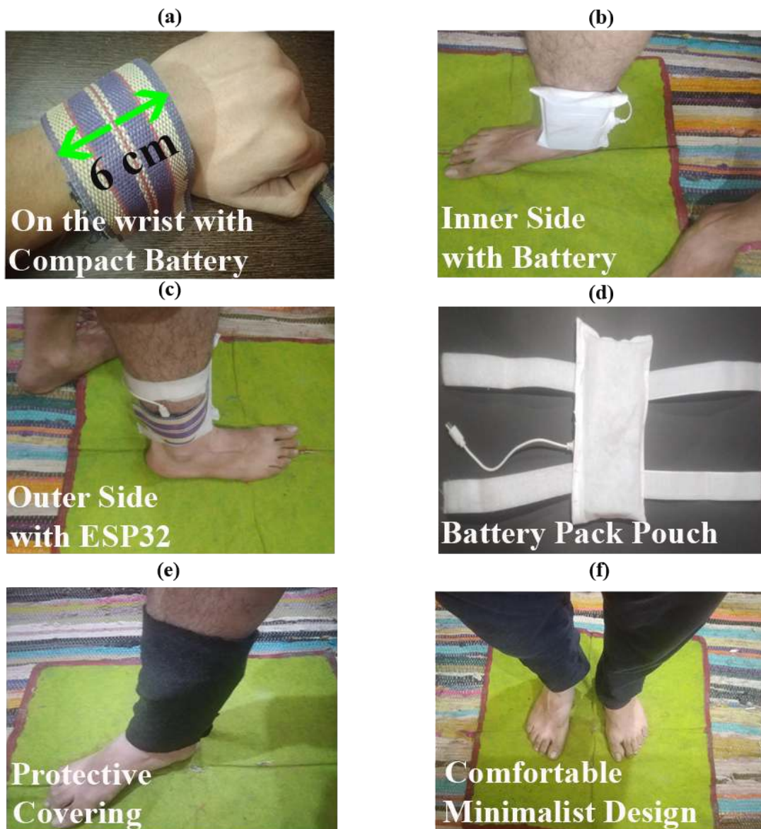
Figure 4. The IoT-Q-Band wearable is comfortably worn over the wrist or leg with firm fitting. (a) Depicts a user wearing the IoT-Q-Band over the wrist. (b) and (c) shows the inner and outer side of the wearable when worn over the legs. (d) shows the battery pouch, whereas (e) shows the protective covering over the IoT-Q-Band so that the band does not hinder the normal walking. (f) shows that even a trouser could be easily worn over the IoT-Q-Band.
