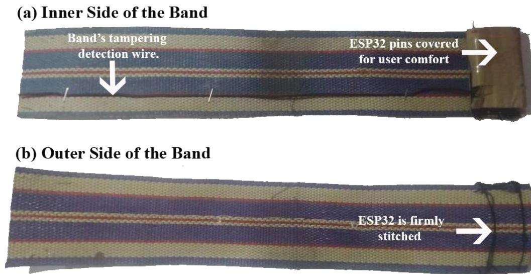
Figure 3. Construction detail of the IoT-Q-Band wearable band showing its construction from (a) inner and (b) outer side.
