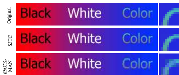
Figure 9: Text compression: Note how black or white text on a colored background works decently for iPACKMAN, whereas our coder has more difficulties with colored text on colored background.
