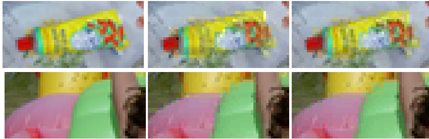
Figure 7: Left: Original. Middle: Images compressed using normal error measure. Right: Images compressed using perceptual error measure. Notice the yellow/white edge (top) and the purple/green edge (bottom). (May look nicer on screen than in print.)
