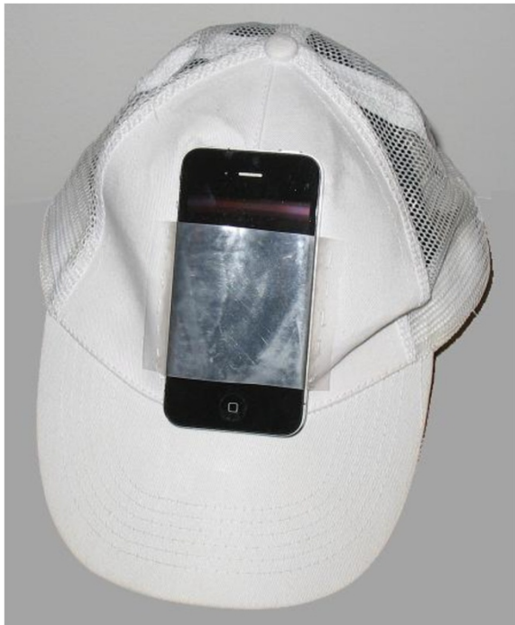
Figure 1 The system design, showing iPod placed in sleeve attached to front of cap.
