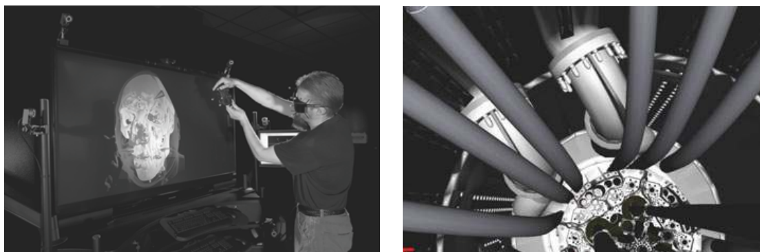
Fig. 3. Left: (a) Here a user manipulates a clipping-plane through computer tomography (CT) data using the Toirt Samhlaigh immersive application. Right: (b) A view looking downward in the ATR reactor vessel. Details shown include: serpentine reactor core, channels and tubes for experiments and large pipes for cooling water.
