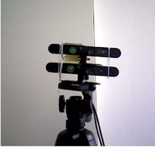
Figure 2. The setup of the Asus Xtion IR image stereo system used in our experiments.
