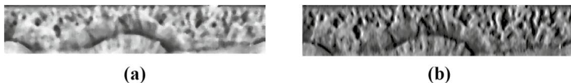
Fig. 4 Image after distortion removal with median filtering (a) and after edges detection with Gabor filter (b)
