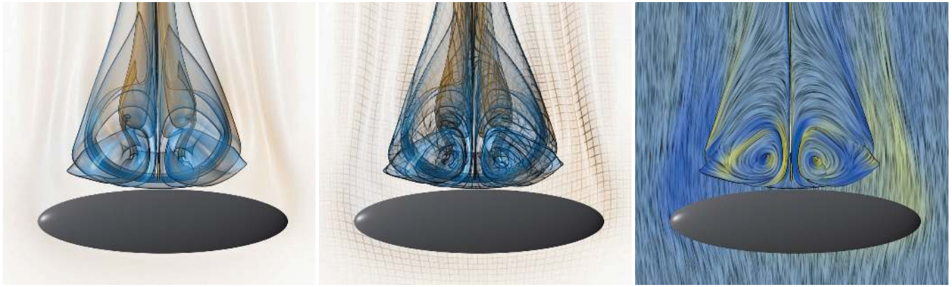
(a) Transparency based on normal variation conveys surface shape. (b) A grid pattern modulating opacity multiplicatively shows both streamlines and timelines. (c) Using a noise texture blurred in t -direction results in a LIC-like depiction of the flow.
