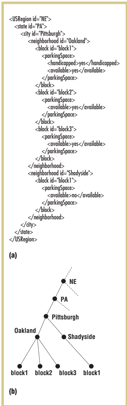
Figure 2. (a) Part of the XML schema used in the parking-space-finder service; (b) the hierarchy defined by the ID-tagged nodes.
