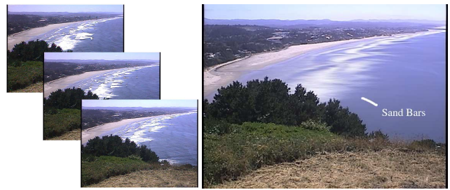
Figure 7: Images from the IRISNET Coastal Imaging prototype. On the left, raw video frames. On the right, temporally smoothed images revealing the sand bars.
