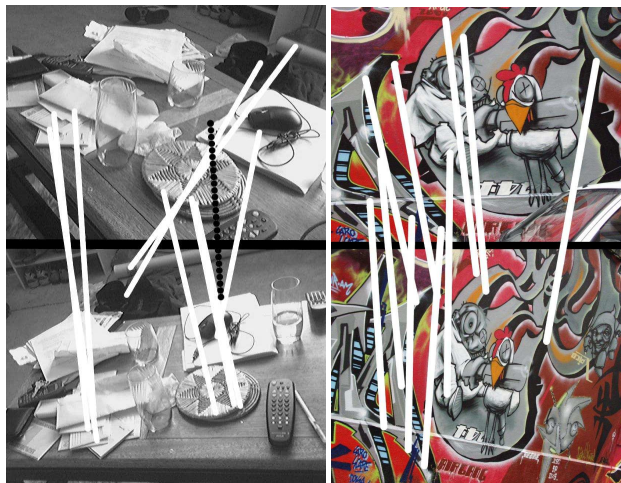
Figure 4: Finding correspondences using PCA-SIFT. Correct correspondences are denoted by white lines and incorrect ones with black dotted lines. 9/10 of the correspondences in the left scene are correct, while 10/10 of the ones in the right scene are correct.
