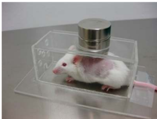
Figure 6. Experimental device to determine the effect of an external magnetic field on the biodistribution of MNPs after i.v. injection into mice in which an inflammatory focus had been induced on their backs. Two \text{Nd}_2\text{Fe}_{12}\text{B} disk magnets, 25 \times 10 mm, of 600 mT per side were placed over the hole in the Plexiglas cages.
