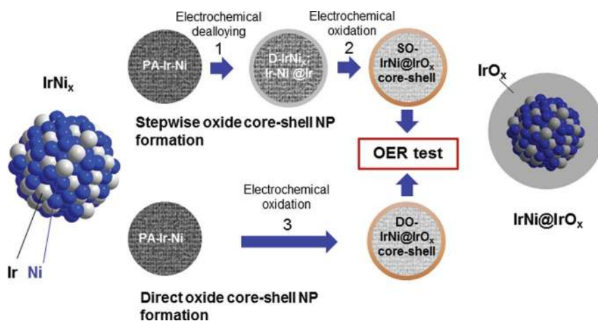
Fig. 1 Synthetic protocol for the preparation of SO- IrNi@IrO_x and DO- IrNi@IrO_x hybrid core-shell nanoparticle catalysts. Precursor IrNi alloys ("PA- IrNi ", and alloy scheme on left, blue: Ni, grey: Ir) are stepwise (SO) or directly (DO) dealloyed and surface oxidized. "D- IrNi_x " denotes the dealloyed stage. The "SO- IrNi_x " or "DO- IrNi_x " nomenclatures emphasize the original stoichiometry of the parent precursor alloy, while the "SO- IrNi@IrO_x " and "DO- IrNi@IrO_x " nomenclature stresses the chemical structure of the core-shell particles.
