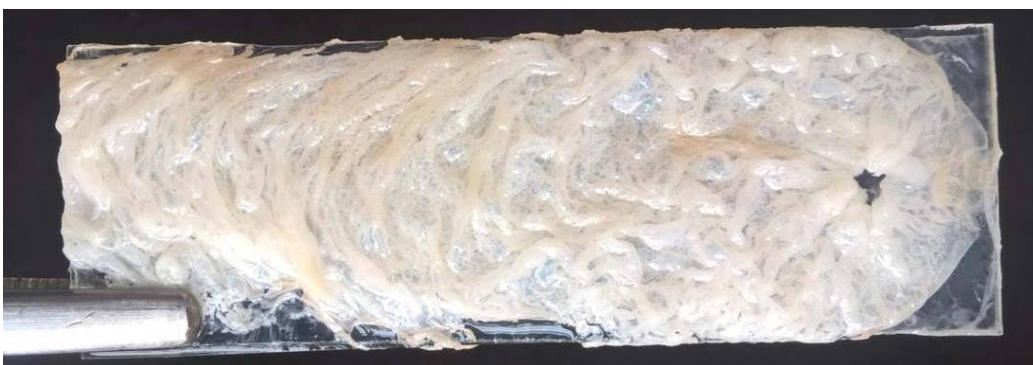
Figure 34: Biofilm after 40 hours of culture in drip flow bioreactor on a PET surface. Biofilm have been fixed to the surface by immersing it in consecutive ethanol solutions of increasing purity.
