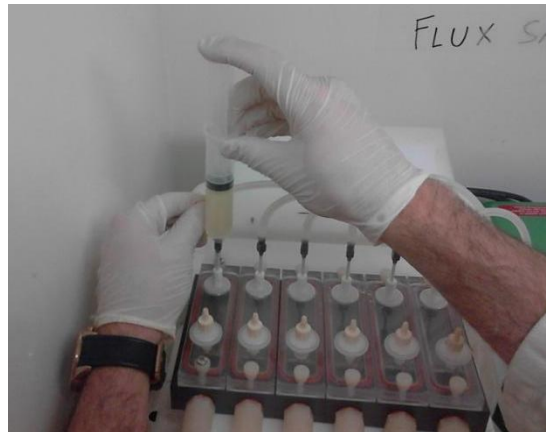
Figure 9: Inoculation of the drip flow chambers with 20 ml of preculture after adjusting its OD to 1 with PBS.
