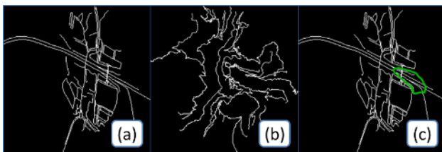
Figure 1. Highway interchange detection in images (a) image with interchange, (b) image without interchange, (c) interchange segmentation.
