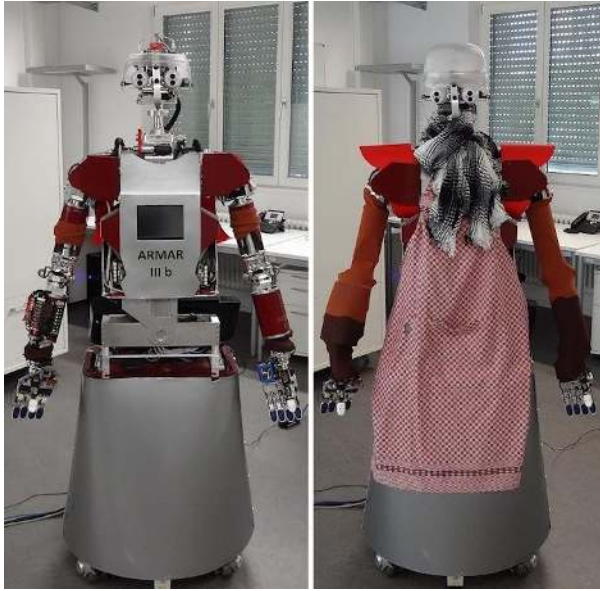
Figure 2. Two different appearances for ARMAR-IIIb: the usual one, with also the head cap removed (left) and the alternative one, wearing human clothes which hide wires and sharp edges (right).
