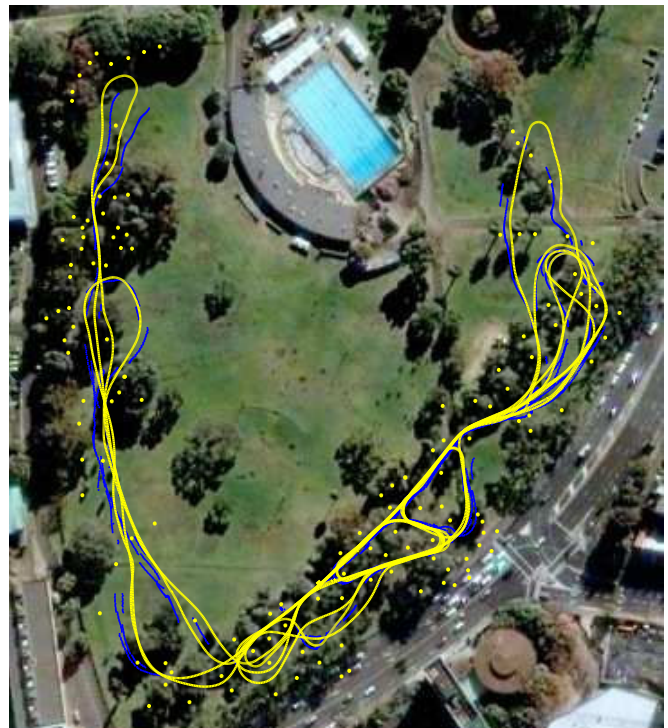
Fig. 8. Optimized map of the full Victoria Park sequence. Solving the complete problem including data association in each step took 4.5 minutes on a laptop. For known correspondences the time reduces to 2.7 minutes. Since the dataset is from a 26 minute long robot run, iSAM with correspondences is over 5 times faster than real time on a laptop computer. The trajectory and landmarks are shown in yellow (light), manually overlaid on an aerial image for reference. Differential GPS was not used in obtaining our experimental results, but is shown in blue (dark) for comparison purposes. Note that GPS is not available in many places.
