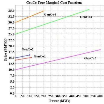
Fig. 4. GenCo true marginal cost functions and true capacity attributes for the benchmark 5-bus test case.
