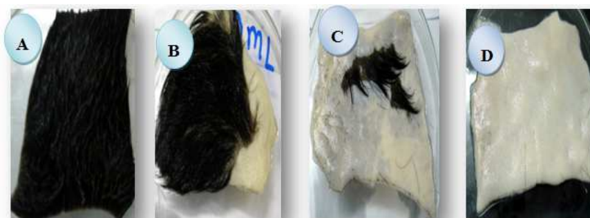
Fig 4. Direct dehairing activity of the enzyme - A (Control), B (10% Hair removed), C (90% Hair removed), D (100% Hair removed)
