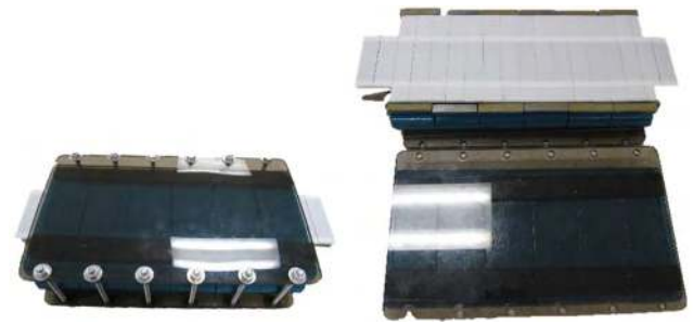
FIGURE 12. Prototype of isolation/filter transformer for 3-Port 3-phase DC-DC converter in Yyd connection.
