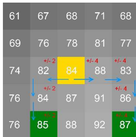
Figure 3: Two-dimensional case of isoline calculation. Blue arrows - best path between the seed (yellow) and a pixel (green). Calculated isoline distance is indicated by red values.
