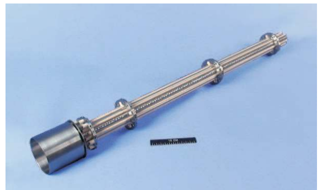
Fig. 17. Photograph of the radiofrequency quadrupole trap used as ion beam cooler and buncher at ISOLTRAP. The electrodes are made of stainless steel and the isolators of glass ceramic (Macor). The indicated scale is 10 cm long.
