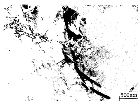
Fig. 17. TEM bright field micrograph taken from a specimen isothermally transformed at 440°C for 40 min, revealing carbide platelets formed in association with the decomposition of a pool of carbon enriched austenite.
