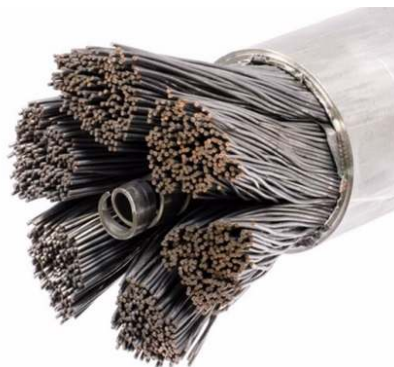
Figure 1-8. Jacketed cable in ITER's toroidal field coil, consisting of superconducting and non-conducting strands around a central channel for helium [117].
