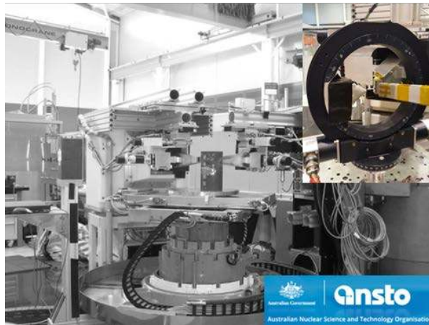
Figure 2-1. KOWARI neutron diffractometer in a general stress setup and texture setup.
