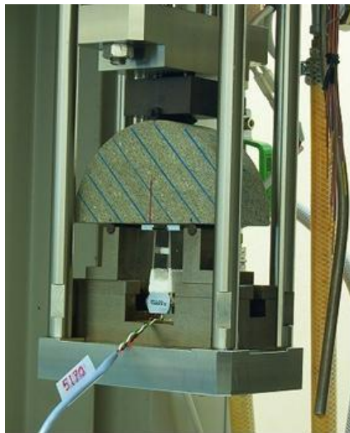
Fig. 3 SCB specimen loading fixture
