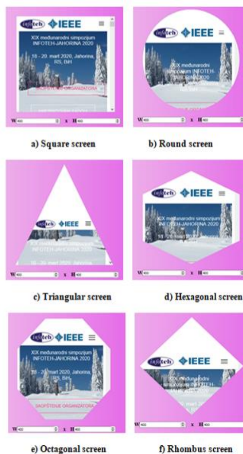
Figure 15. The corrected layout of the Infoteh – Jahorina symposium web page using the responsive testing tool
