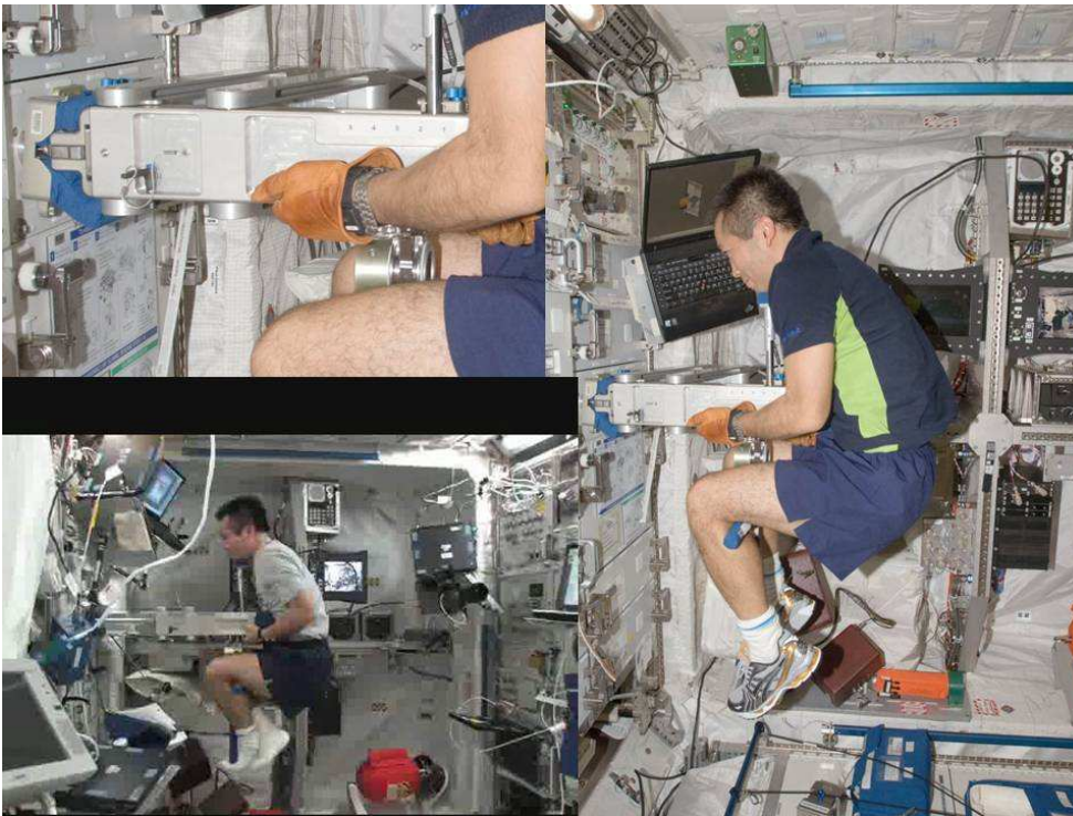
Fig. 13. NASA SLAMMD. Japanese astronaut Koichi Wakata weighs himself with the Human Research Facility's Space Linear Acceleration Mass Measurement Device (SLAMMD) on ISS, 2009.
