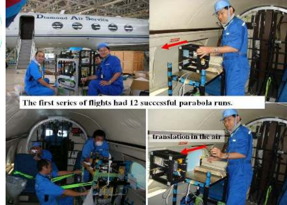
Fig. 18. Dummy mass parabolic flight test.
