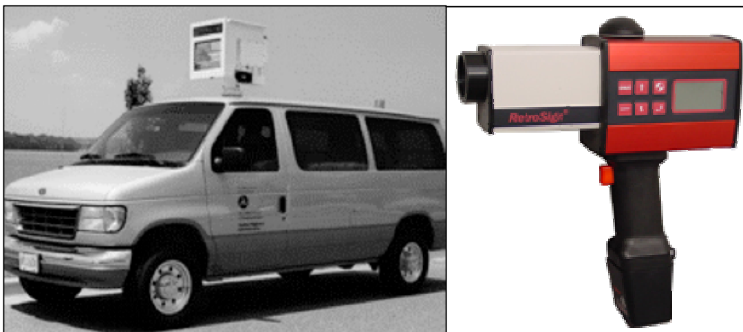
Figure 4. Sign Retroreflectivity Measurement: FHWA SMARTS Van and Handheld Retroreflectometer
