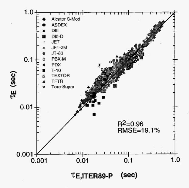
Fig. 3 Total energy confinement time plotted as a function of the ITER89-P scaling. The line corresponds to τΕ=τΕ,ITER89P.
