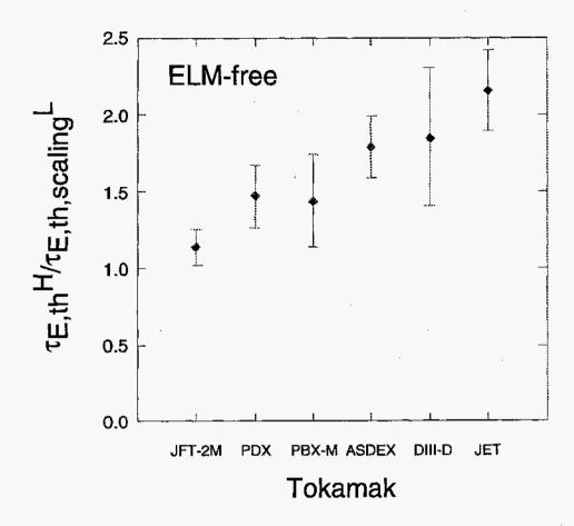
Fig. 10 Ratios of the ELM-free H-mode thermal confinement time to that of the L-mode scaling. The error bars correspond to the standard deviations of the ratios.
