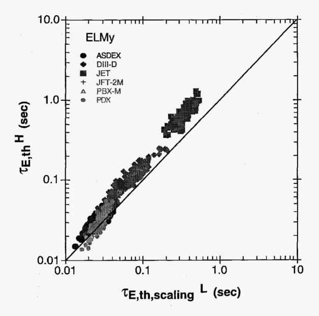
Fig. 7 Thermal experimental energy confinement time of the standard subset of ELMy discharges in the H-mode database plotted as a function of the L-mode thermal confinement time scaling value. The line indicates \$\tau\_{E,th}^{H}=\tau\_{E,th}\$, scaling \$L\$.
