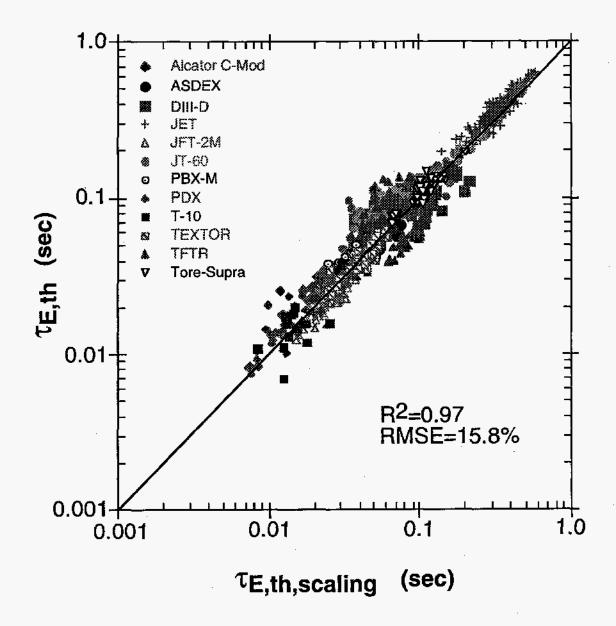
Fig. 6 Thermal experimental energy confinement time plotted as a function of the scaling value. The line indicates  $\tau_{E,th}=\tau_{E,th,scaling}$
