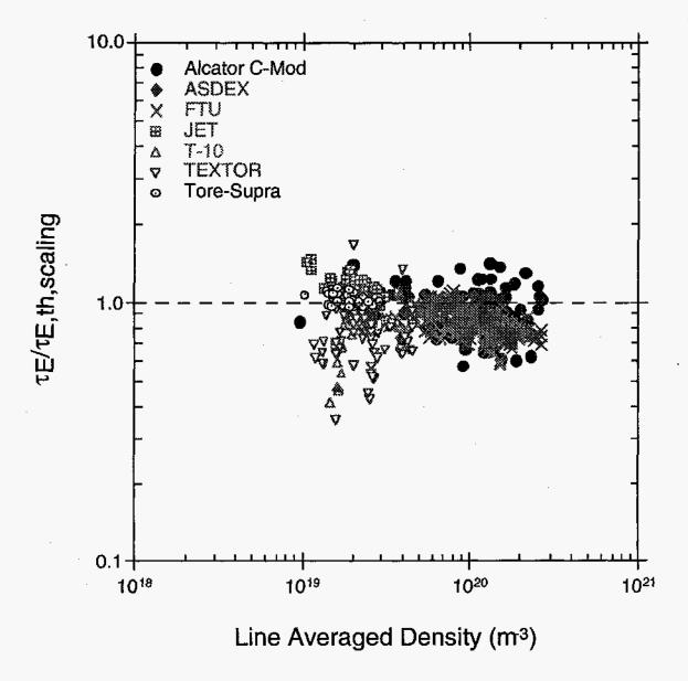
Fig. 2 Ratio between the measured energy confinement time and that of the scaling given in Eq. 8 for the deuterium subset of ohmic database versus line averaged density.
