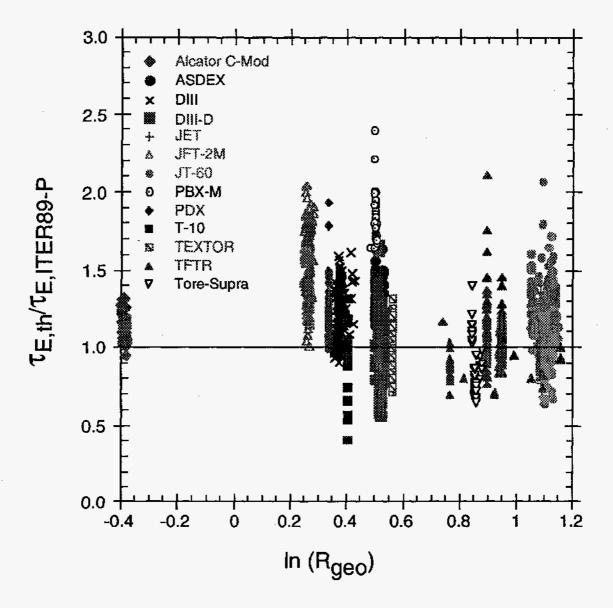
Fig. 4 Ratio of the total energy confinement time relative to that given by the ITER89-P scaling for each device.
