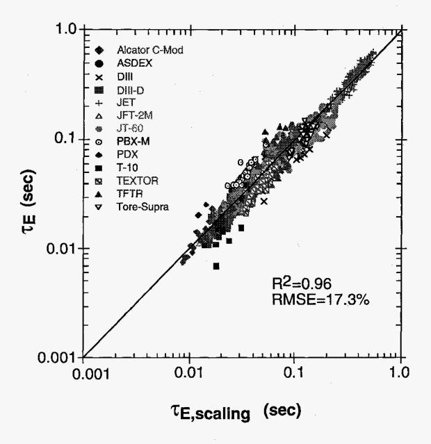
Fig. 5 Total experimental energy confinement time plotted as a function of the scaling value. The line corresponds to τ<sub>E</sub>=τ<sub>E,scaling</sub>.
