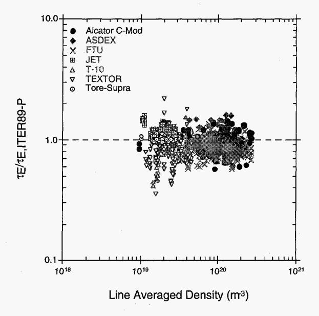
Fig. 1 Ratio between measured energy confinement time and that of the ITER89-P scaling for the deuterium subset of ohmic database versus line averaged density.
