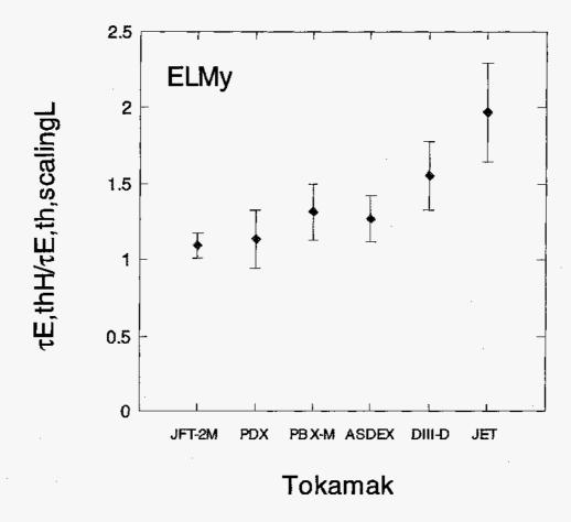
Fig. 8 Ratios of the ELMy H-mode thermal confinement time to that of the L-mode scaling. The error bars correspond to the standard deviations of the ratios.
