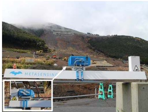
Fig. 1. The deployed GB-SAR system.
