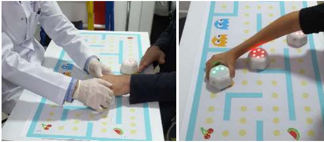
Figure 1: Gamified upper arm rehabilitation with tangible robots. Therapist can hold the patient's hand and easily assists the game play if needed.
