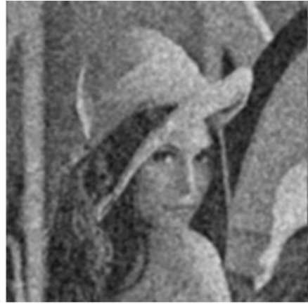
(b) Intermediate residue obtained after subtracting IFD mode 1 from original image in Figure 16(a). Signal-to-noise level for this image is 17.1 dB.
