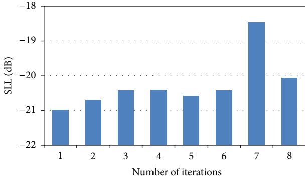
FIGURE 2: Number of iterations in relation to SLL with the target SLL of \leq -20 dB.
