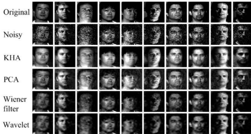
Fig. 6. Face image denoising based on PCA and KHA with 256 PCs, Wiener filter, and wavelet from Matlab. The SNR value was 7.58dB, 8.29dB, 8.45dB, and 8.31dB, respectively.
