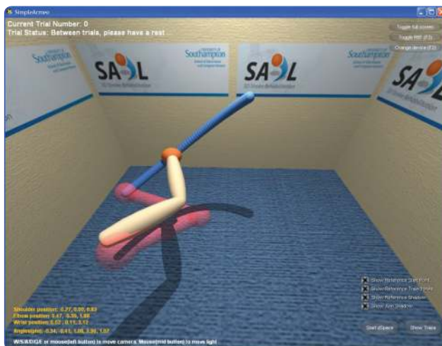
FIGURE 16 Three-dimensional virtual reality environment for patients, showing reaching trajectory comprising a sphere moving along a path and a graphic of the arm. Visual feedback provided by changing sphere color.
