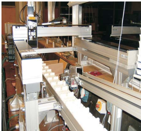
Fig. 3. Illustration of the gantry robot.
