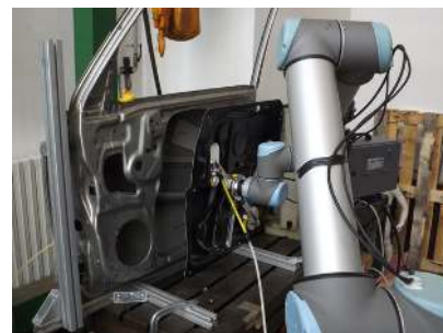
Fig. 1: Experimental set-up. A Universal Robot UR 10 involved in the assembly of the target automotive component.
