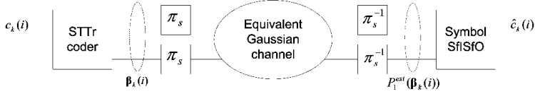
Fig. 5.3. Block diagram of an STTr coded system.
