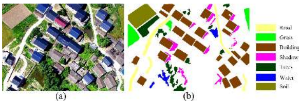
Fig. 6: UAV image. (a) Three-band false-color image and (b) ground reference map and class legend.
