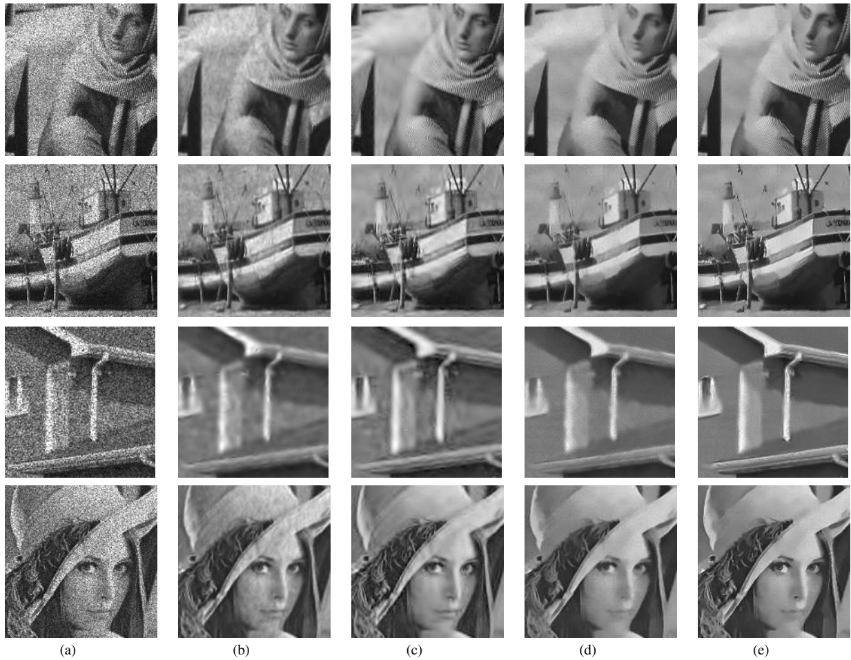
Fig. 4. (a) From top to bottom, corrupted images of Barbara , Boat , House and Lena by a multiplicative speckle noise with equivalent number of looks L = 3 . Denoised images using (b) the WIN-SAR filter, (c) the MAP-UWD-S filter, (d) our non-iterative PPB filter and (e) 25 iterations of our PPB filter.
