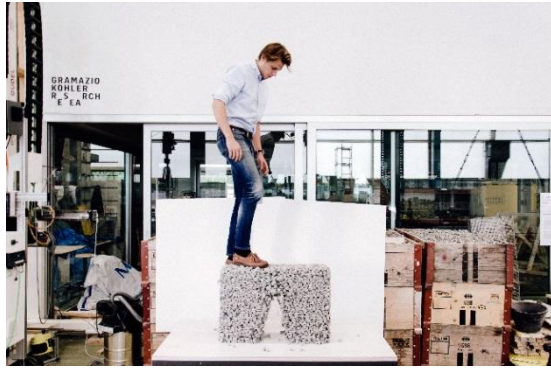
Fig. 3 A structurally sound wall element made with jammed, low-grade, granular materials. Gramazio Kohler Research, ETH Zürich, 2014.
