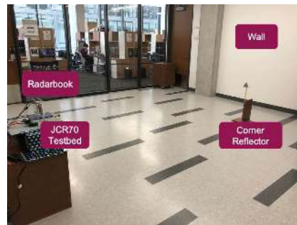
FIGURE 8. Experimental set-up to evaluate the radar performance of our testbed for a single-target scenario using a corner reflector in the indoor lab.
