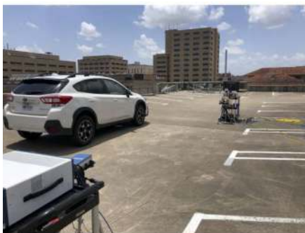
FIGURE 17. Outdoor JCR measurement scenario using a car on the top of a parking garage. The cart with the JCR70 transmitter and radar receiver is kept in front of the car, whereas the cart with the JCR70 communication receiver is kept behind the car.
