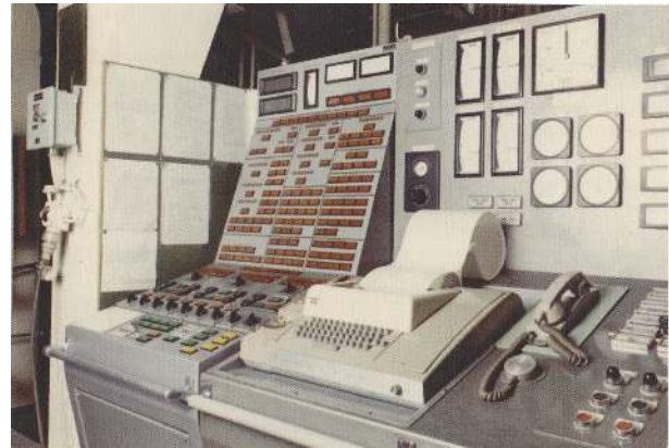
Figure 8: A prototype of a computer-based ship automation system onboard the M/S Taimyr. Courtesy of Kongsberg Maritime.
