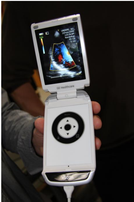
Figure 12: Vscan is a pocket-sized ultrasound machine from GE Vingmed Ultrasound in Horten. Photo: Camilla Aadland.
