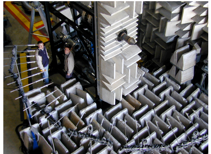
Figure 2: The Small Hot Jet Acoustic Rig (SHJAR) located in the Aero-Acoustic Propulsion Laboratory (AAPL) at the NASA Glenn Research Center (GRC) shown in acoustic configuration with the 24-microphone array located on a 150-inch radius arc centered on the nozzle exit.
