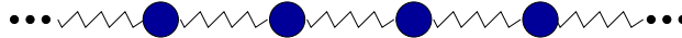
Figure 5. The model of discrete elasticity considered in §3. The atoms are coupled to their neighbours by nonlinear springs.
