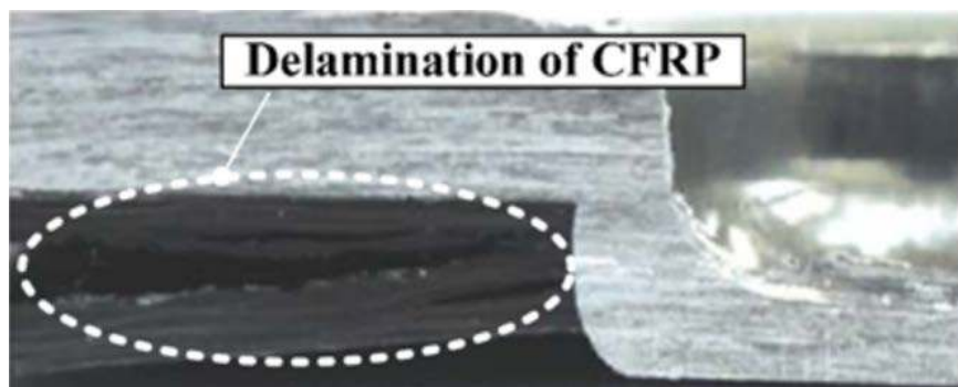
Fig. 35: Delamination of CFRP laminates in hole-clinched joints [117].
