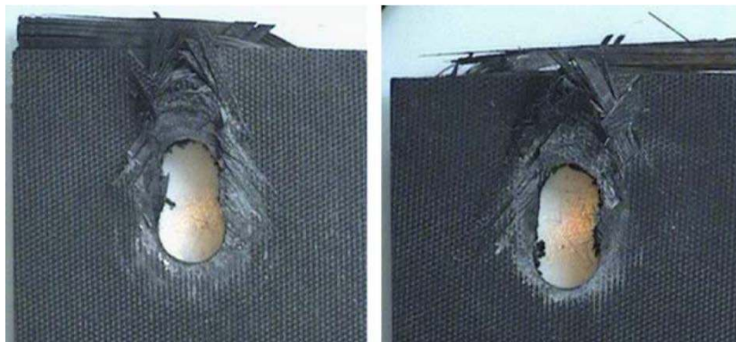
Fig. 26: Laminates after bearing failure of bolted joints [97].
