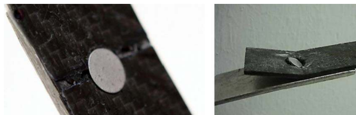
Fig. 22: Failure types of SPR joints with (a) CFRP cross-ply and (b) CFRP angle-ply [77].
