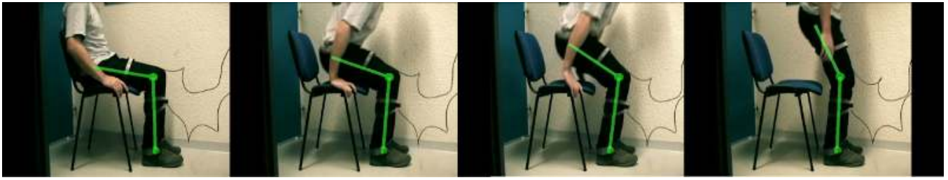
Fig. 2. Angles estimated using inertial sensors in a sit-to-stand task.
