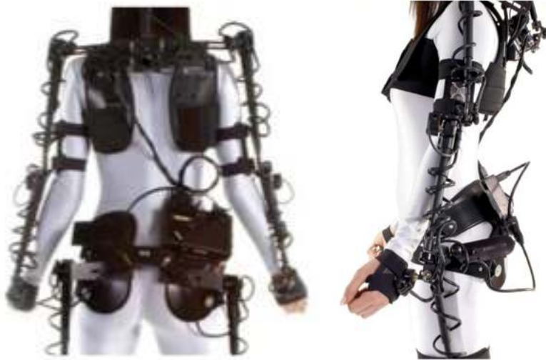
Figure 1.2: Example of mechanical sensor device (Gypsy). An electromechanical suit manufactured by Animazoo that contains a combination of 37 potentiometers and 2 gyroscopes. Published with permission from Animazoo UK Ltd, Brighton, UK.
