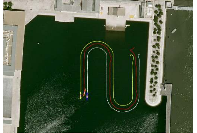
Fig. 7. Aerial view of the mission area and trajectory (real data). The maneuver starts on the top right corner, and the trajectory of the controlled vehicle is shown in red.
